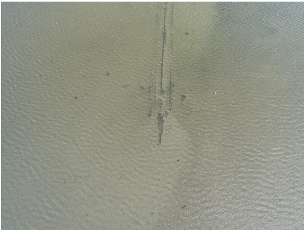
Figure E-6. Jet plow track showing start of jet plow. For scale, the combined width of the two skids are approximately 15 ft wide. 4:13 PM, Sept 9, 2019.
